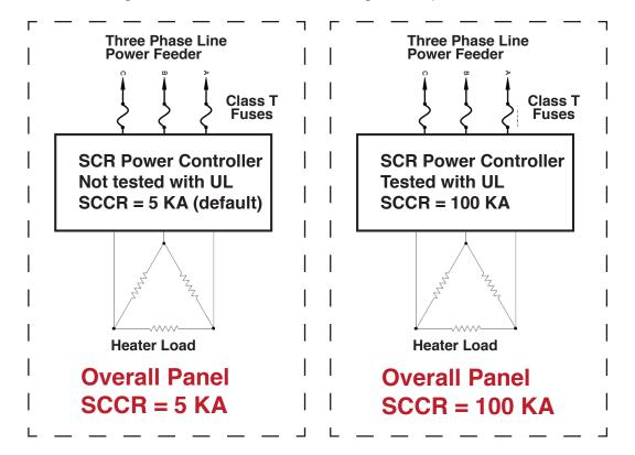
Control Concepts FUSION / Compact FUSION series of SCR Power Controllers are UL certified to 100 KA SCCR - much above the 5 KA default value.
