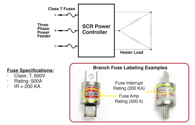
In accordance with NEC409, in order to safely connect directly to the feeder circuit, the panel must be designed for a <u>minimum</u> SCCR of 100 KA. So far, the design appears sound. The feeder circuit Fault Current is 100 KA and the fuse IR of 200 KA exceeds that value, as required. At this point, an erroneous assumption is often made: The panel SCCR = fuse IR = 200 KA. This is not necessarily true!
