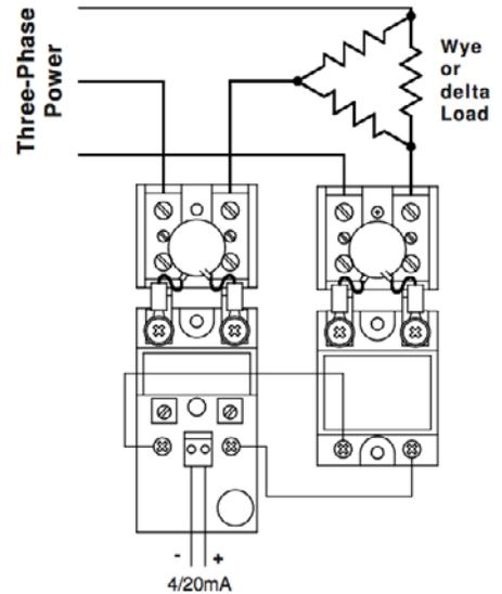
The model 3020 control circuit is powered by the current loop command signal. It does not require a transformer
