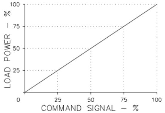
3 electrical cycles and OFF for 3 electrical cycles. At lower power levels load power is applied for 3 cycles and the number of OFF cycles is increased.
