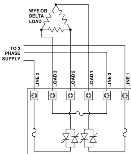
Due to internal space limitations, Units rated 425 Amps or more do not have internal line fuses. It is recommended that the user install fuses in the power lines ahead of the controller. Size the fuses at about 125% of the maximum current load.
