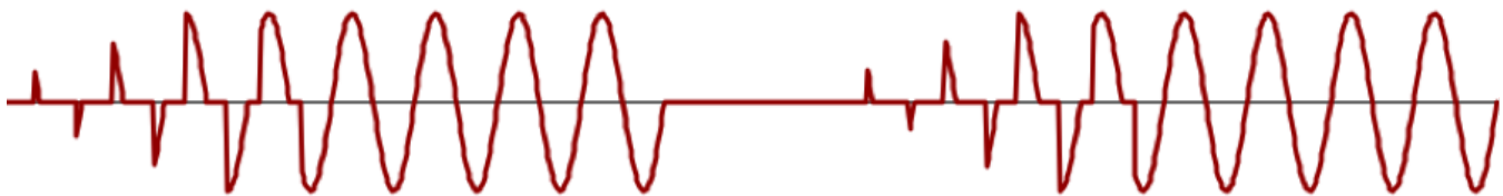
Figure 4: Zero Cross Transformer Mode
