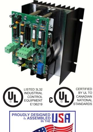
The model 1032A is a single-phase, phase-angle SCR power controller that features either RMS voltage control or RMS current control, user adjustable RMS current limiting or voltage limiting, soft start with missing cycle detection and line voltage compensation.
