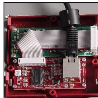
Ferrite placed as close to the cable end as possible.
