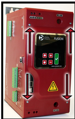
Figure 3.00: Remove (4x) screws
