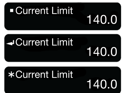
Figure 4.01: Top - Unlocked Settable Parameter, Middle - Selected Parameter, Bottom - Locked Parameter
